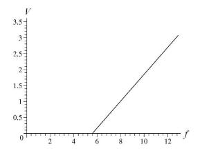
(b) Our least squares fit procedure can also determine the *y*-intercept for that line. The *y*-intercept is the negative of the photoelectric work function. In this way, we find  $\Phi = 2.31$  eV.
